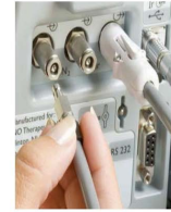
Connect gas supply line to delivery system port on the back of the unit.
