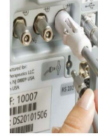
Purge gas supply line
