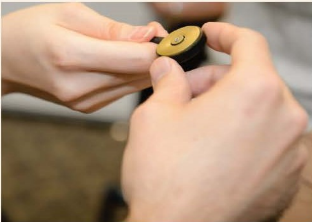
THIS TACTOR, SIMILAR TO THE TECHNOLOGY THAT MAKES A CELL PHONE BUZZ, IS DESIGNED SO THAT RIGGS CAN MANIPULATE PARAMETERS LIKE AMPLITUDE, FREQUENCY, AND PULSE PATTERN.
