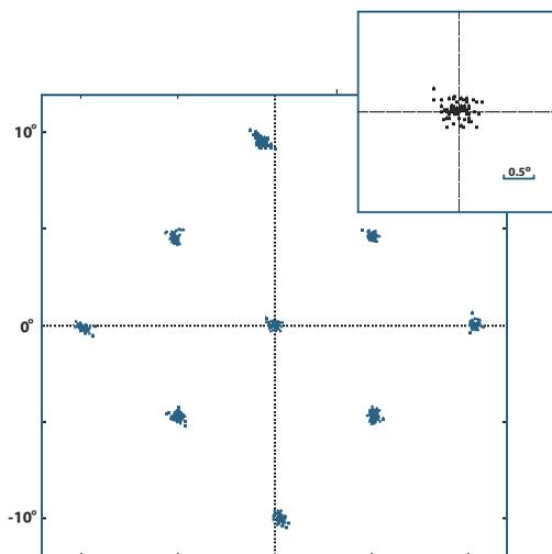
Accuracy was assessed without a head support using the Remote Camera Upgrade. Repeated target fixations to nine screen locations resulted in the low error levels demonstrated by the fixation error histogram below (Mean = 0.41°, Median = 0.40° and Standard Deviation = 0.22°). The inset plot is an enlarged view of the fixation distribution around the center target position. See Page 4 for analogous data using head-stabilized tracking.
