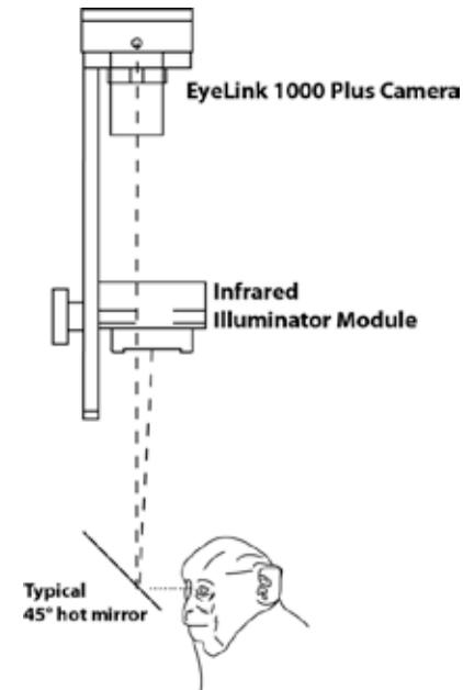
The EyeLink 1000 Plus eye tracker outputs eye position and pupil size data in either digital or analog formats. Both outputs can be linearly calibrated using the built-in offset and gain adjustments. The gain and offset adjustment states can be saved and reloaded at a later date, allowing for easy switching between participants.
