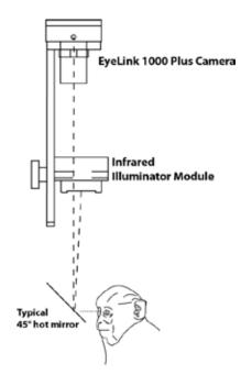
The EyeLink 1000 Plus eye tracker outputs eye position and pupil size data in either digital or analog formats. Both outputs can be linearly calibrated using the built-in offset and gain adjustments. The gain and offset adjustment states can be saved and reloaded at a later date, allowing for easy switching between participants.
