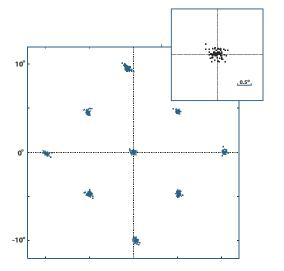
Accuracy was assessed without a head support using the Remote Camera Upgrade. Repeated target fixations to nine screen locations resulted in the low error levels demonstrated by the fixation error histogram below (Mean =  $0.41^{\circ}$ , Median =  $0.40^{\circ}$  and Standard Deviation =  $0.22^{\circ}$ ). The inset plot is an enlarged view of the fixation distribution around the center target position. See Page 4 for analogous data using head-stabilized tracking.
