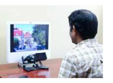
Head distance is accurately measured at up to 1000 Hz using a small target sticker allowing head compensation even during blinks, and providing an extremely fast 1 msec blink recovery time.
