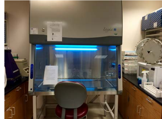
Laminar Flow Hood for PBMC Processing and Aseptic Methods
