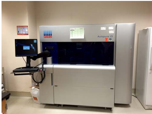
Qiagen Autopure for Large Volume Automated DNA Extraction
